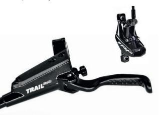
For E-MTB touring riders who are looking for stability and reliability. From the outside it differs by its brake lever design, but from the inside it is on the same level of performance as the DHR EVO. A 10 mm lever piston provides easier modulation for control over long descents.
