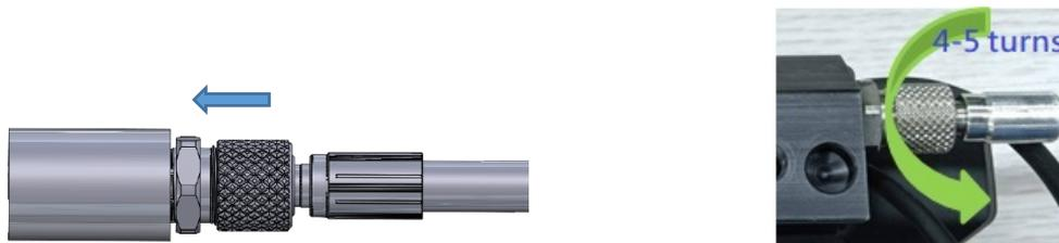
1. Push the union nut towards the ABS unit and plug the hose connector into the union nut at the same time.
