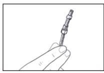
C-1 Install cap, nut and olive before installing the barb!
