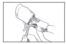
B-1 Tighten clamp nut with 5mm hex wrench
