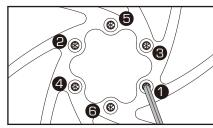
A-1. Rotor torquing sequence
